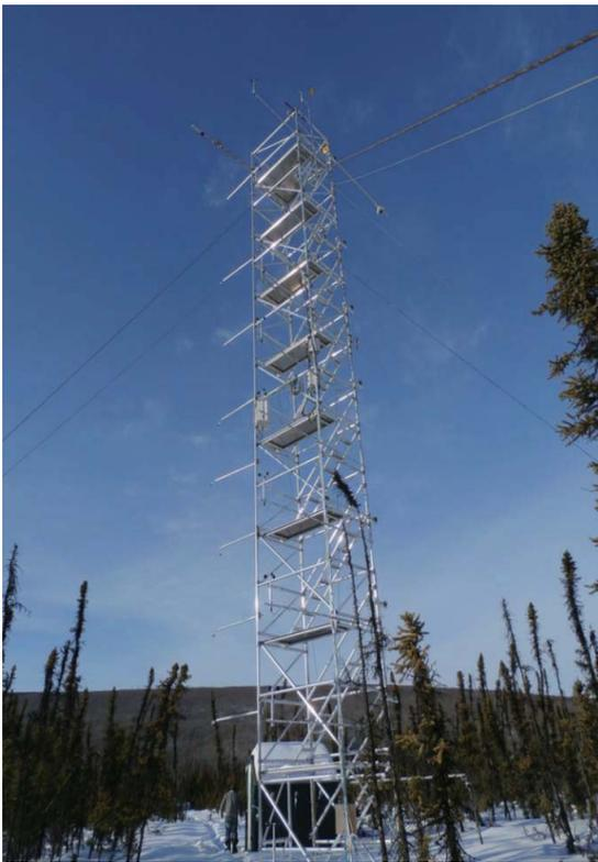
**Fig. 3.** The 17m scaffold tower for eddy covariance and micrometeorological measurements in the black spruce forest in the property of the Poker Flat Research Range.
