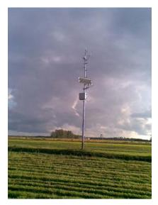
Figure 11. Micrometeorological station for momentum and virtual sensible heat surface flux measurements.
