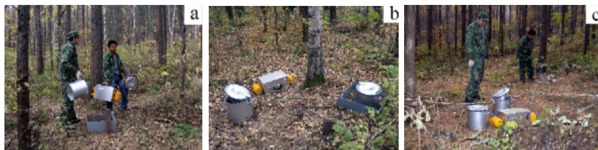
Fig. 4 Application of the portable automated chamber system for measuring soil CO 2 efflux in a larch forest in northeast China.
