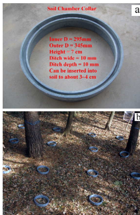
Fig. 2 A collar with ditch can be used for attaching tight to the chamber (a) and collars are installed at the forest floor (b).
