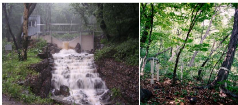
Fig. 4 Weir (left) and stem flow and through fall measuring systems for hydrological research.
