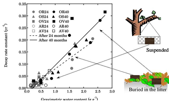
**Figure 4. Relationship between decay-rate constant and gravimetric water content of the block specimens**
