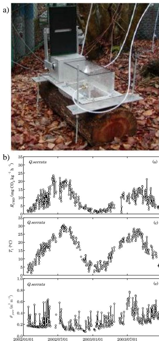
**Figure 2. Automatic operated measurement system (a) and the seasonal changes in CWD respiration ( $R_{CWD}$ ), temperature (TCWD), and water content of CWD ( $\theta_{pore}$ ).**
