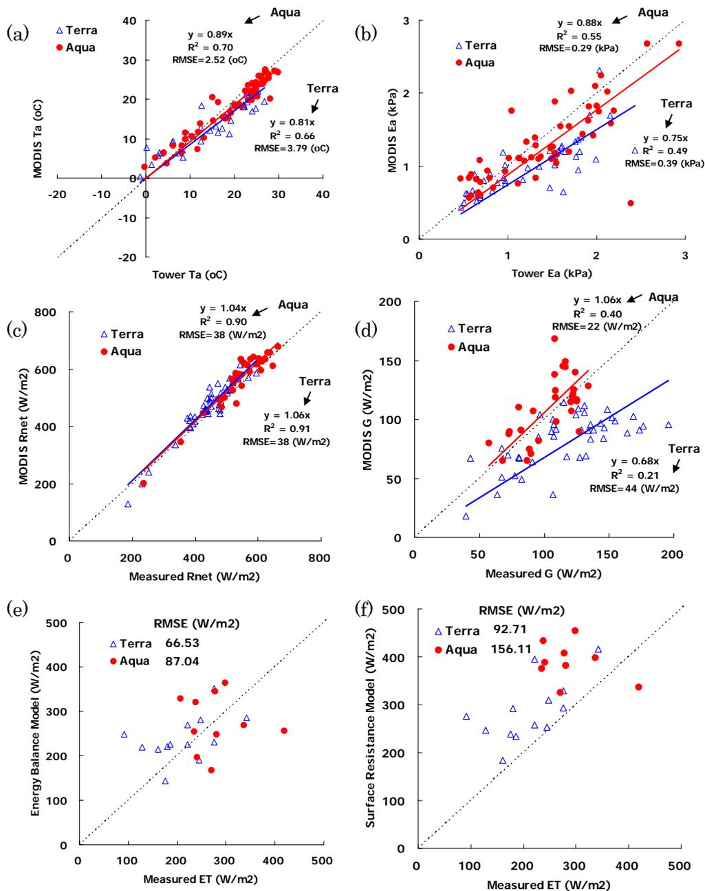
Figure 2. Comparisons between estimated/extracted and measured variables for (a) surface layer air temperature extracted from MOD07, (b) surface layer vapor pressure extracted from MOD07, (c) net radiation estimated by using both MODIS and flux tower data, (d) ground estimated by using MODIS data, (e) ET estimated by using the modified Penman-Monteith model, and (f) ET by using the modified Priestly-Taylor model, respectively.
