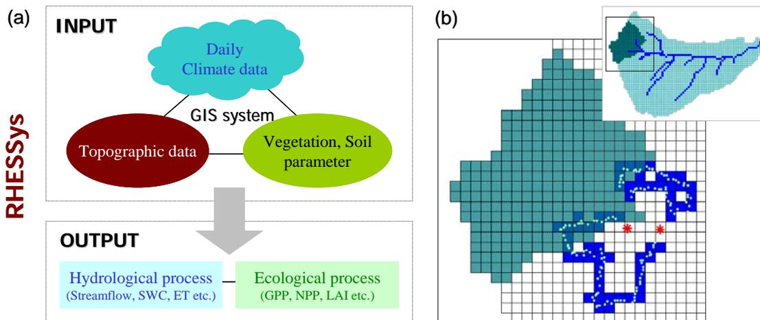
Figure 3. Schematic diagrams on RHESSys and study area: (a) key input and output variables of RHESSys and (b) the GRF watershed (upper right key map) and sampling points for soil water content (dots in right figure). Pixel size is 30 m × 30 m and the asterisk indicates flux tower location.
