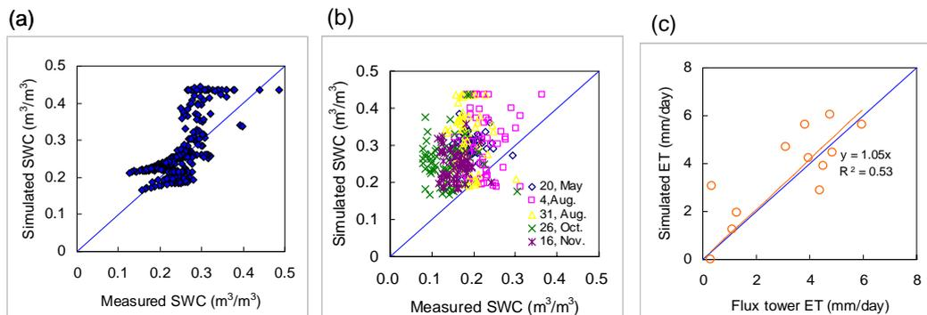
Figure 4. Comparisons between measured and simulated soil water content: (a) daily mean soil water content in 2002 (RMSE = 0.06 m³/m³), (b) transect measurements of soil water content in 2005 (RMSE = 0.13 m³/m³) and (c) daily ET of flux tower point in 2002 (RMSE = 1.25 mm/day).
