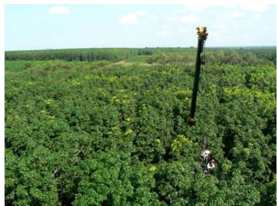
Fig. 6 Leaf gas exchanges measurements with a crane.
