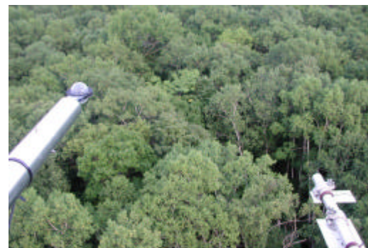
The netradiometer on the left side and the sensors for reflective solar radiation and PPF on the right side, above the canopy of Sapporo Forest Meteorology Research Site.
