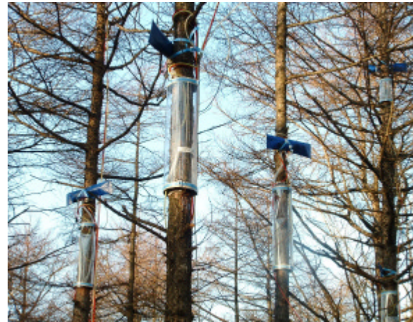
Fig.4 Overview of field measurement of woody tissue respiration with the multichannel automated stem-chamber system at Tomakomai flux site.
