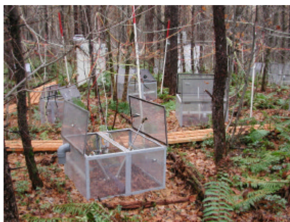
Fig.1 Overview of field measurement of soil CO 2 efflux with the multichannel automated soil-chamber system at Tomakomai flux site.
