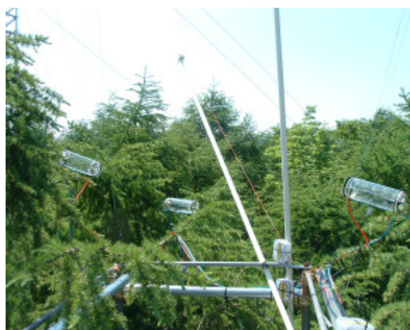
Fig.6 Overview of field in situ measurement of shoot-level photosynthesis with the multichannel automated branch-chamber system at Tomakomai flux site.
