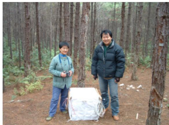
**Photo. 2 Static chamber used within ChinaFLUX for measurements of CO<sub>2</sub>, CH<sub>4</sub>, and N<sub>2</sub>O emissions from the soil.**
