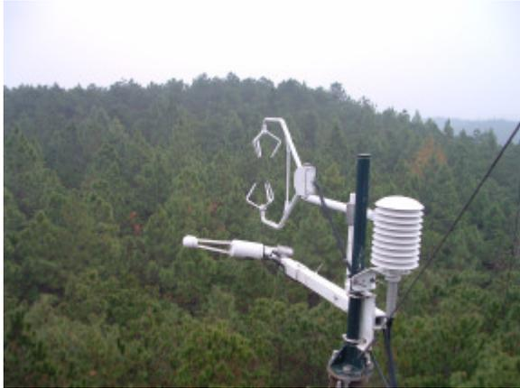
**Photo. 1 Eddy covariance measurement system on the flux tower of Qianyanzhou Station.**
