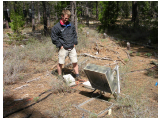
Photo. 3 Automated soil CO 2 efflux chamber designed by James IRVINE.
