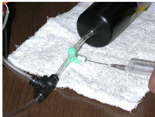
Fig. 2 Photograph of the CO 2 sensor response experiment under the diffusion condition.
