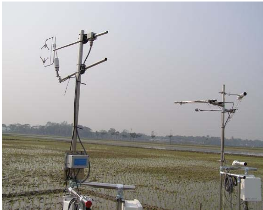
Fig. 3. Sensors for eddy covariance flux measurement (left) and those for meteorological components (right).
