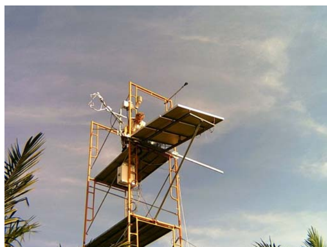
Fig. 4 The eddy correlation instrument tower established in an oil palm plantation at Sintok, Kedah.
