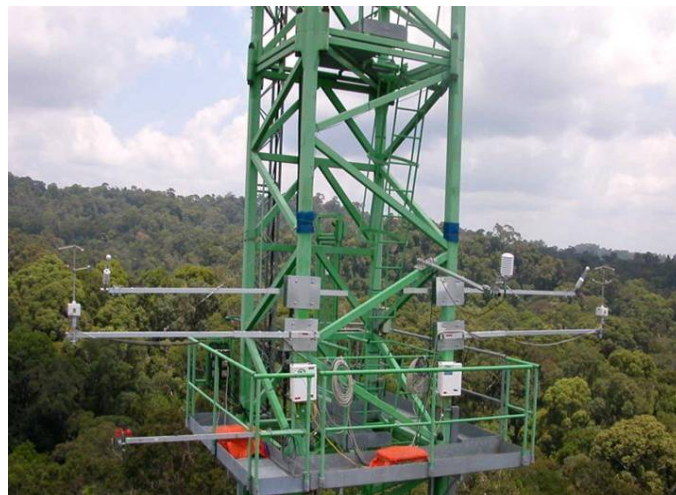
Fig. 3 Flux observation system on the 80m crane established at Lambir Hills National Park, Sarawak.
