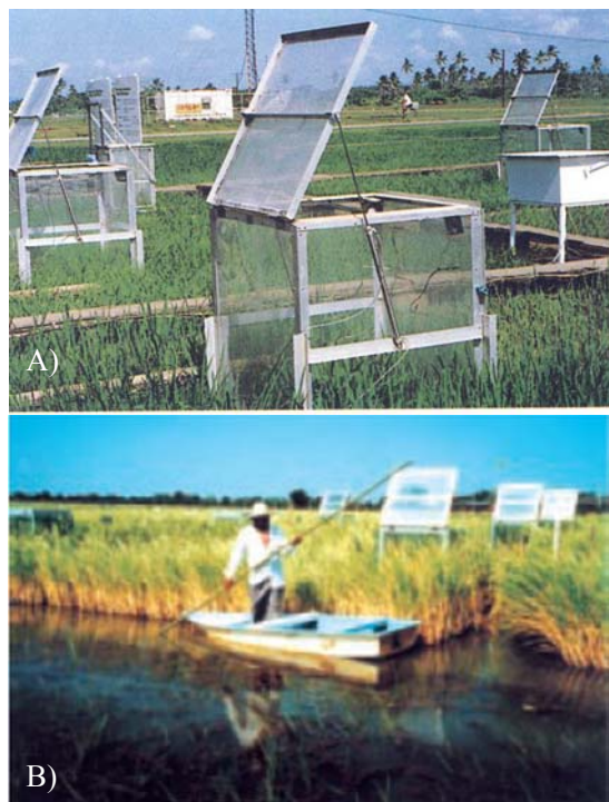
Fig 3 Methane emission field chambers under irrigated conditions (A: IRRI, Philippines) and under deepwater conditions (B: Prachinburi, Thailand)
