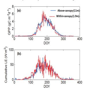
**Fig. 4.** (a) Daily gross primary productivity (g C  $m^{-2} d^{-1}$ ) and (b) latent heat flux (W  $m^{-2}$ ) measured within the black spruce canopy were 80% and nearly 100% of those measured above the canopy. Data were obtained in 2011 at the black spruce forest site in the Poker Flat Research Range.
