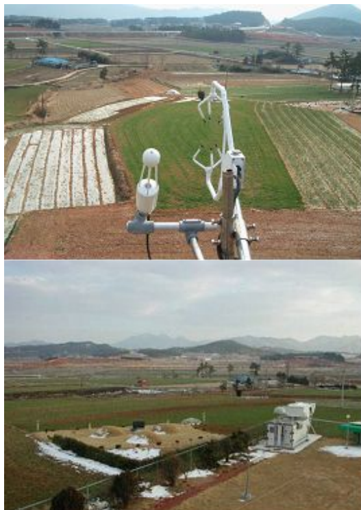
Fig. 2 Eddy covariance system (top) and Autosonde (bottom) of Haenam site.
