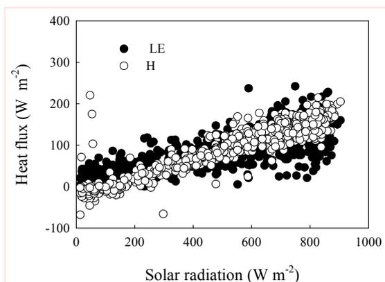
**Fig. 4 Relationship between latent heat (LE)/sensible heat (H) and incoming solar radiation during daytime in August, 2006 at site L. Site L stands for the site at the lower elevation in the wetland.**
