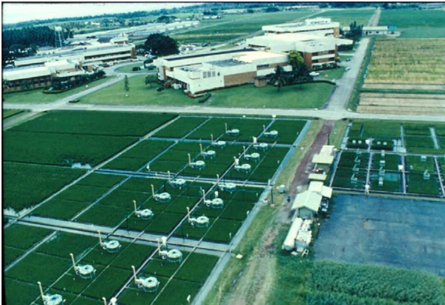
Figure 2. The open-top CO 2 chambers (left side), the automatic closed chamber for CH 4 measurements (right side), and the IRRI research centers (at the back) which house the gene bank with 110,000 rice accessions
