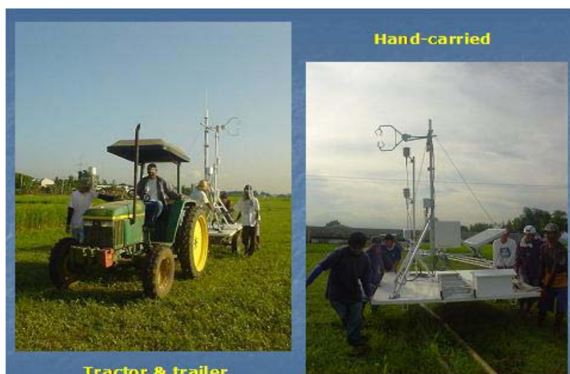
Fig. 6. Transporting the eddy covariance system
