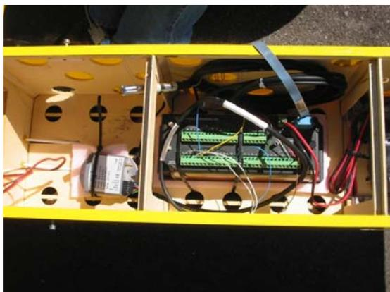
Figure 2. Sensor and datalogger layout inside *Aerolemma-1*.
