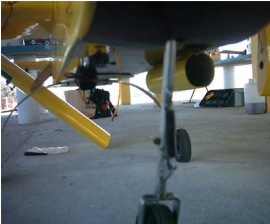
Figure 4: External shield for housing the temperature sensor
