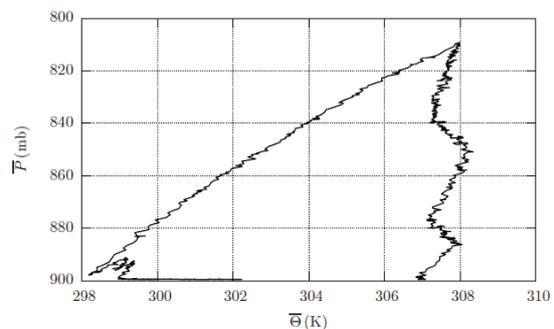
Figure 3. Hysteresis on the temperature measurements due to sensor positioning inside the fuselage
