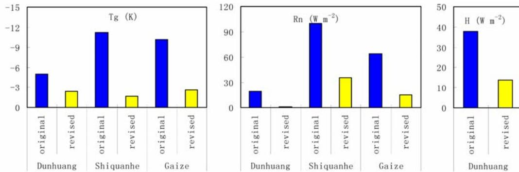
Figure 5. Mean biases of the original Noah model and the revised one for three dry sites during the daytime (0900-1600 LT), calculated from 30-minute observations and simulations. Sensible heat flux was not observed at Shiquanhe and Gaize sites (Courtesy of Dr. Yingyi Chen).
