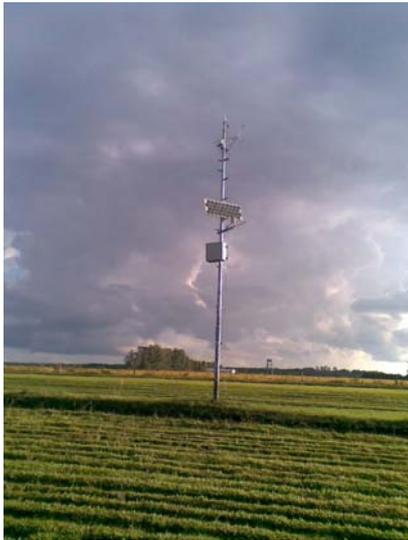
Figure 11. Micrometeorological station for momentum and virtual sensible heat surface flux measurements.
