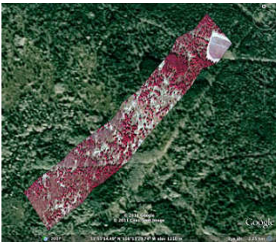
Figure 7. False color infrared image (red stripe overlaid on top of Google Earth) from a helicopter flight over the boreal forest near Hinton, Alberta, in May 2010. Note the clear resolution of individual tree crowns (in red), illustrating the high spatial resolution (approx. 20 cm) possible with airborne imaging spectrometry. Carbon flux can be derived from spectral reflectance (invisible Z dimension of the image) using the LUE model. Image centre location approximately 53°55'14.44"N, 116°13'31.36"W, elev. 1209m. Unpublished data, J. Gamon (University of Alberta) and D. Stonehouse (VeriMap Plus, Calgary, Alberta), using an imaging spectrometer (MicroHyperspec, Headwall Photonics, Fitchburg, Massachusetts).
