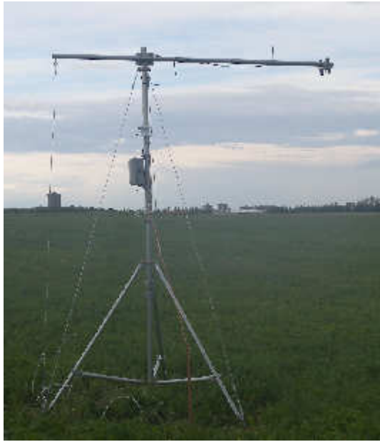
Figure 3. “Phenology station” sampling NDVI using simple, 2-band radiometers in an alfalfa field (Edmonton, Alberta, Canada). Shown here is a system sold by Onset Computer Corporation (Bourne MA, USA), but many brands of these sensors now exist. These stations can be operated alone, or linked into an expandable global network using satellite links. When properly calibrated against eddy covariance, phenology station sensors can provide reliable estimates of biospheric carbon uptake, and can be used to fill gaps in flux measurements (figure 4). The stations can also be compared to aircraft and satellite sensors (figure 8) to validate remotely sensed products, and enable wider regional extrapolation of carbon flux measurements.
