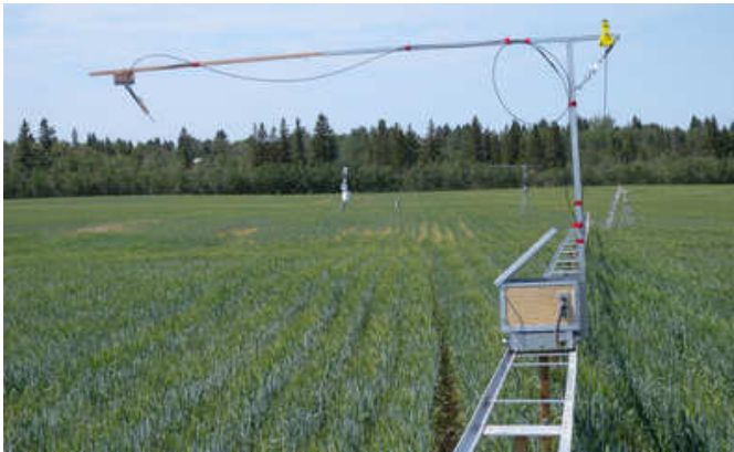
Figure 6. Sampling surface reflectance in a flux tower footprint using a tram system (Gamon et al. 2006b) in a barley ( Hordeum vulgare ) field (Edmonton, Alberta, Canada). Note that the spectrometer foreoptic can be pointed at different directions, allowing multi-angle sampling. Similarly, by sampling at different times of day, reflectance can be sampled at different sun angles.
