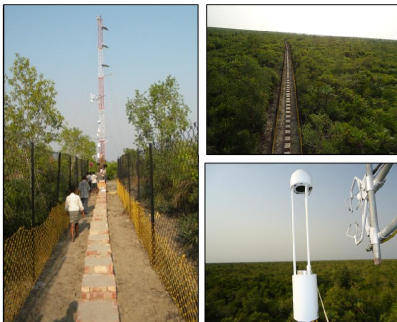
Fig. 3: EC Flux tower with surrounding canopy cover and fast response instruments at the Sundarban Biosphere Reservoir site.
