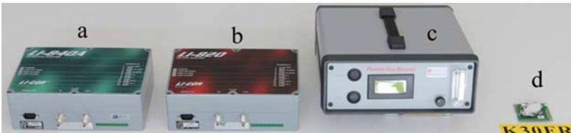
Fig.2. Non-dispersive infrared CO<sub>2</sub> analyzers can be used by LAC. a: LI-840 (Li-Cor); b: LI-820 (Li-Cor); c: PGA (ADC); d: K30FR (SenseAir).
