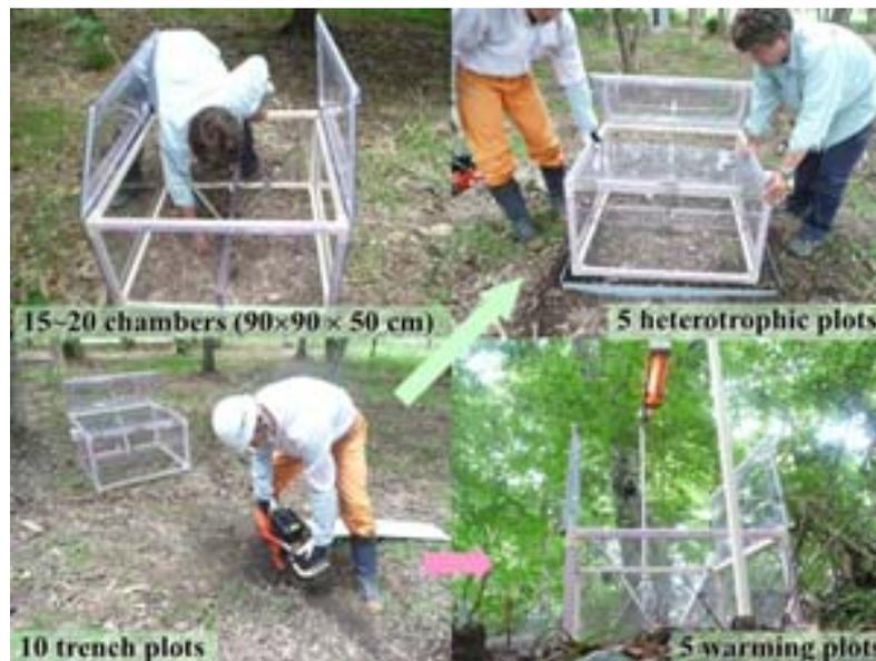
Fig.16. A multichannel LAC applied in a soil warming experiment.
