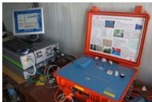
Fig.15. A multichannel LAC coupled with both CO<sub>2</sub> and isotopic CO<sub>2</sub> analyzers for measuring NEP and isotopic CO<sub>2</sub> flux at a Mongolian arid grassland site.
