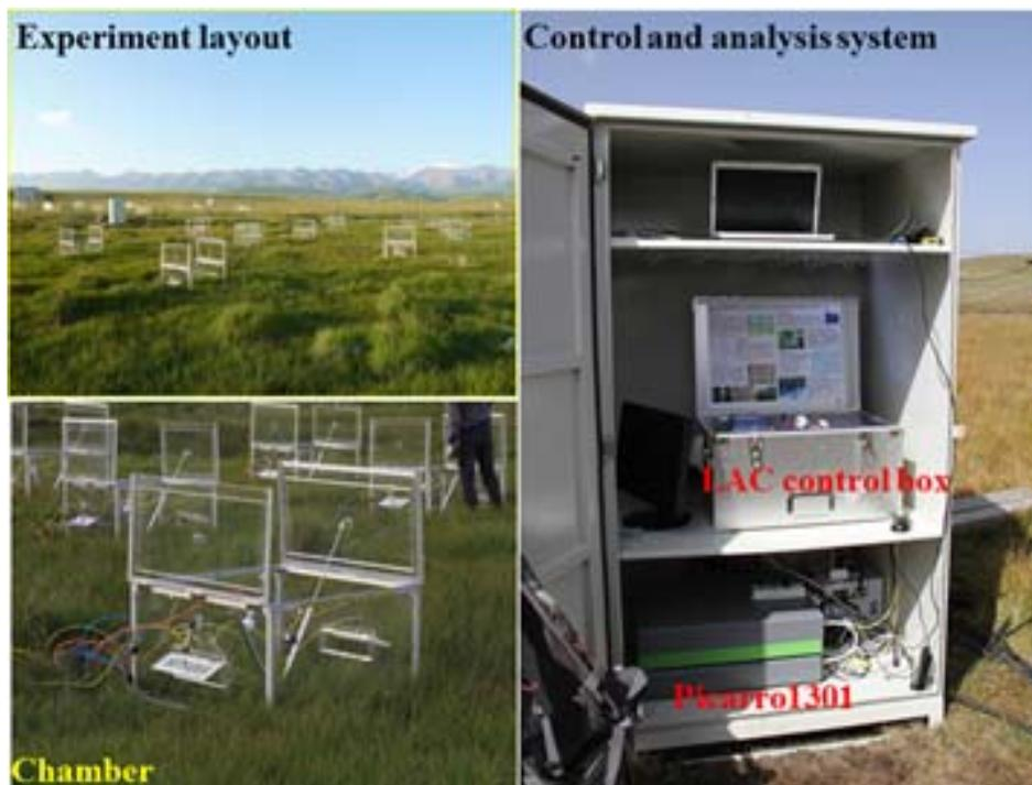
Fig.14. A multichannel LAC coupled with both CO<sub>2</sub> and CH<sub>4</sub> analyzers for measuring CO<sub>2</sub> and CH<sub>4</sub> fluxes at a wetland on Tibet Plateau.
