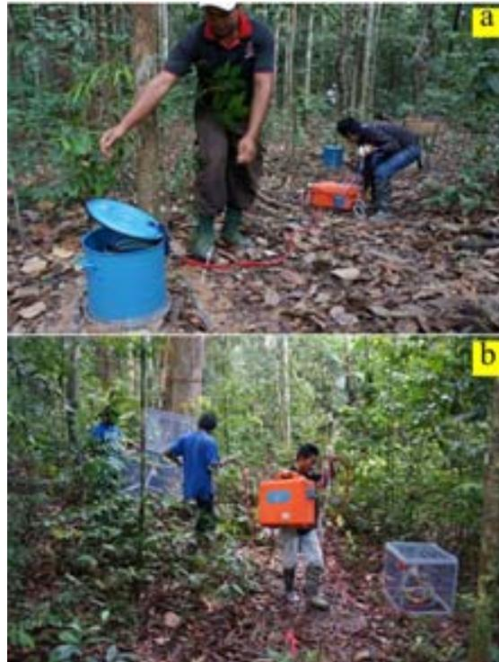
Fig.13. Measuring spatial variations of soil respiration using portable LAC at a secondary forest (a) and primary forest (b) in Pasoh of Peninsular Malaysia.
