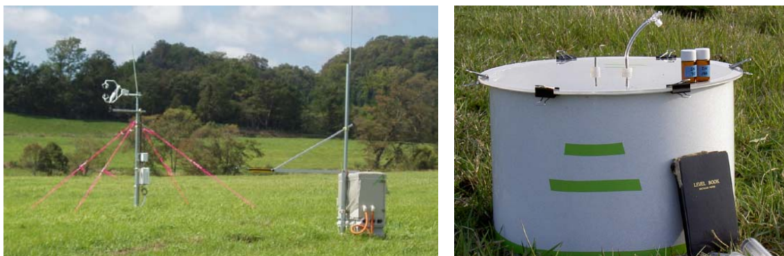
Figure 2. Sets up for measuring CO 2 by an eddy-covariance technique (left) and CH 4 and N 2 O by chamber method (right)
